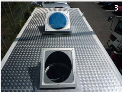
Photo 1. LIDAR (two containers on the left) and FTS (container on the right) set up right next to the Building 7 (four story building in the back) at Saga University. Photo 2. LIDAR installed inside the container. Photo 3. Two observation windows built in the roof of container (the one in the back is for tropospheric ozone LIDAR, and the one in the front is for aerosol observation). Photo 4. The sky radiometer (left) and sky camera (right) on the rooftop of the Building 7. Photo 5. JAXA's high resolution FTS installed inside the container. Photo: 1 Shuji Kawakami (JAXA) 2-5 Osamu Uchino
