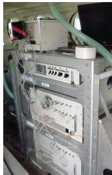
Photo 2. The laser instrument for CO 2 measurement installed on the airplane. The instrument measures the amount of CO 2 between the airplane and the ground by emitting the near-infrared laser light through the window and by receiving the diffused light that comes back after being reflected on the ground with a telescope. Photo: Daisuke Sakaizawa
