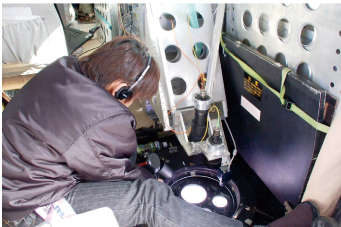
Photo 1. On the airplane, the writer (Sakaizawa) warming up the window with a hairdryer to keep it from being fogged. Photo: Diamond Air Service Inc. (DAS)
