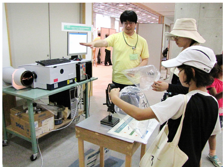
An experiment to measure CO 2 in a plastic bag using an instrument similar to the sensor on "IBUKI." NIES Special Researcher Yukio Yoshida explaining to the visitors.
