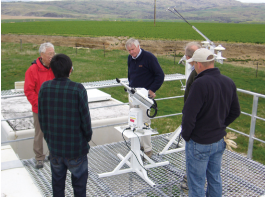
Photo 3. A Skyradiometer installed on the rooftop of the Optics Laboratory of the Lauder Atmospheric Research Station. Photo by Tomohiro Nagai.
