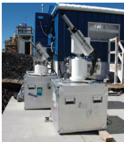
Image 1. The Skyradiometers (POM-02) and two Sun Photometers installed for calibration data acquisition at the MLO.
