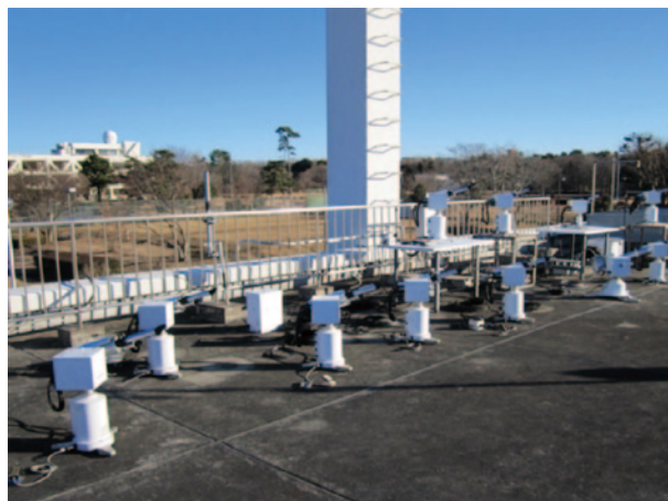
Image 4. Cross Comparison of the Skyradiometers at the Meteorological Research Institute (transferring calibration constants).
