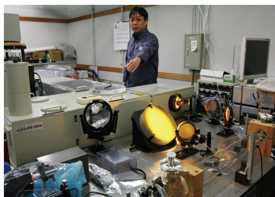
NIES Senior Researcher Isamu Morino demonstrates the high-resolution FTS installed in the Atmospheric Minor Constituents Spectra Observatory in the Climate Change Research Hall at NIES. The sunlight comes into the observatory through a hole on the roof, and then reflected by the gold mirror into the FTS. In the FTS, the spectrum of sunlight that was affected by the absorption by greenhouse gases is measured.
